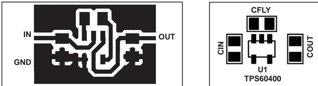
Figure 37. Recommended PCB Layout for TPS6040x (top layer)
