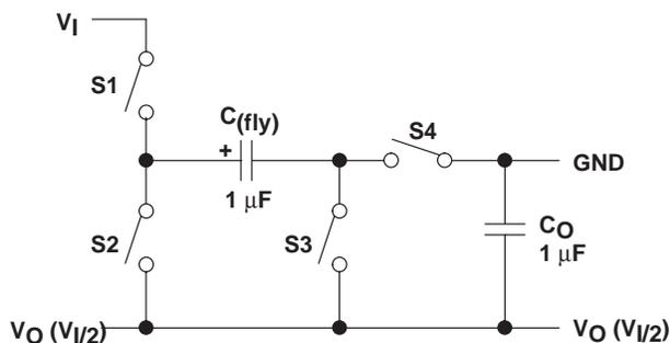
Figure 34. Step-Down Principle
