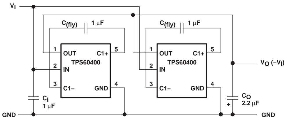
Figure 29. Paralleling Devices
